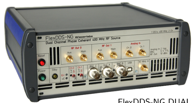
FlexDDS-NG DUAL Dual Channel Standalone RF Generator
