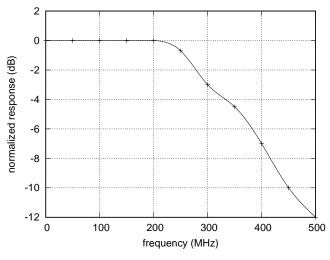
Test conditions: Light input 100  $\mu\mathrm{W}$  at 1310 nm, modulated via EOM.
