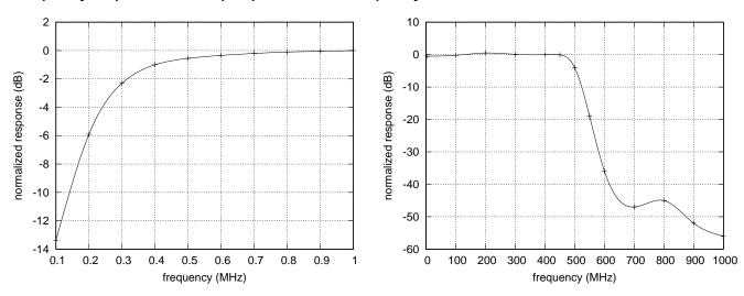
Test conditions: Light input 100  $\mu$ W at 1550 nm, modulated via EOM.
