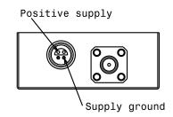
Supply connector (front view). The case is electrically connected to ground. There are two types of supply cable, one has 2 wires (new cable) and one has 5 wires (old). The corresponding color scheme of these cables is:
