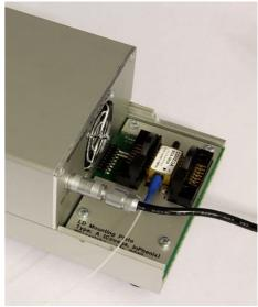
The laser diode is mounted directly at the back of the WL-LDC10D. Different slot-in mounts for different pinouts are available.
