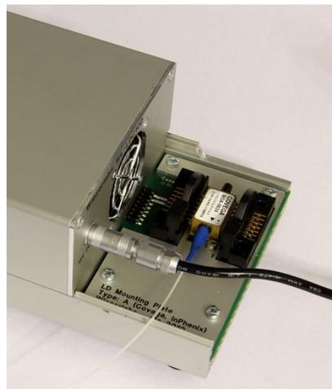
The laser diode is mounted directly at the back of the WL-LDC10D. Different slot-in mounts for different pinouts are available.
