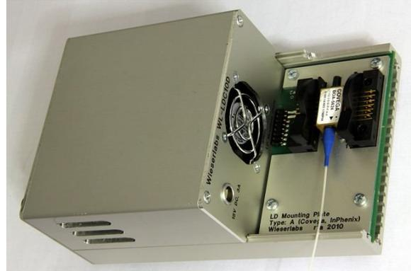
Note: The screws ensure that the butterfly package has good thermal contact with the aluminum LD mounting plate for heat sinking.
