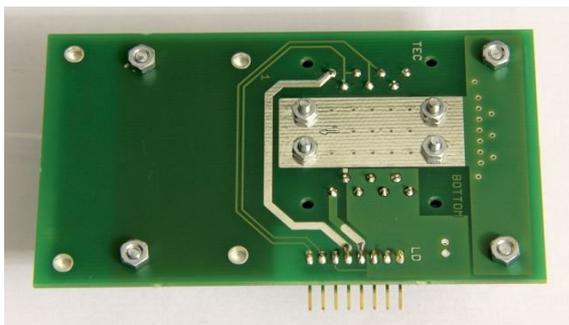
screw driver, mount the nuts from the bottom side onto the screws and fix them firmly.
